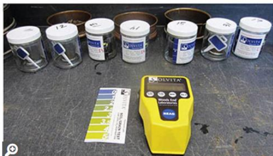
Fig. 1 Solvita® soil test equipment and supplies; color chart, color reader, soil beakers and gel indicators in air-tight jars.
